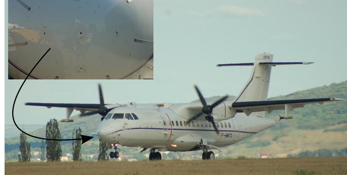
five pressure sensors on the radome of the aircraft nose measure the air velocity in the aircraft reference frame; the wind vector is estimated by subtracting the aircraft velocity with reference to the ground (from navigation system
