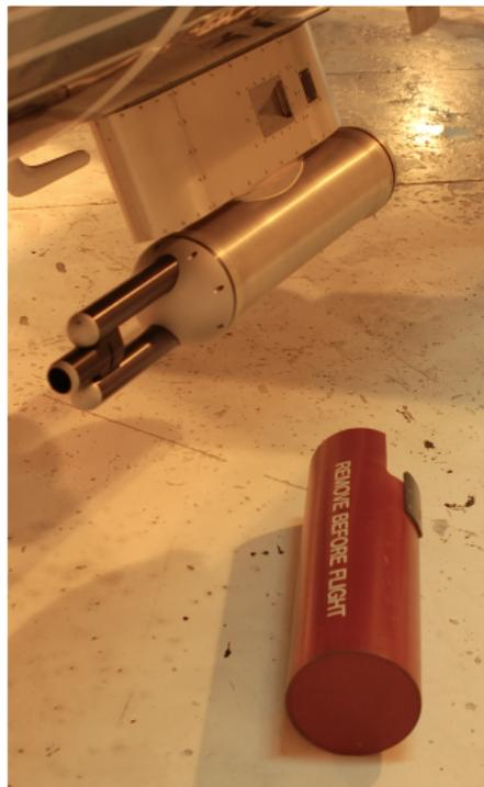
(FSSP under the SPEC Learjet fuselage)
