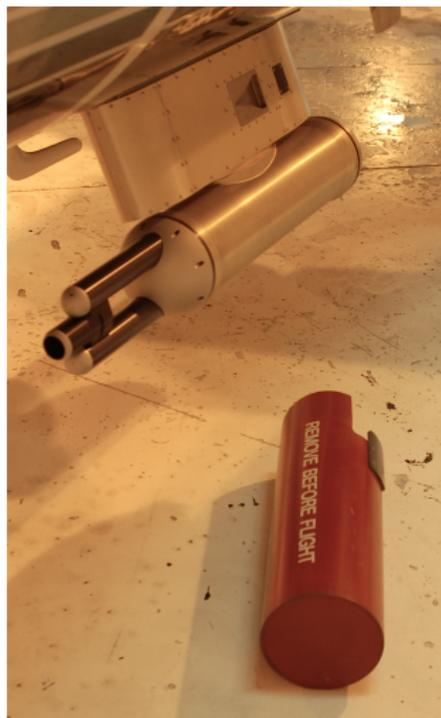
(FSSP under the SPEC Learjet fuselage)
