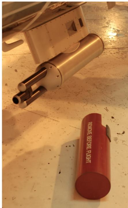
(FSSP under the SPEC Learjet fuselage)
