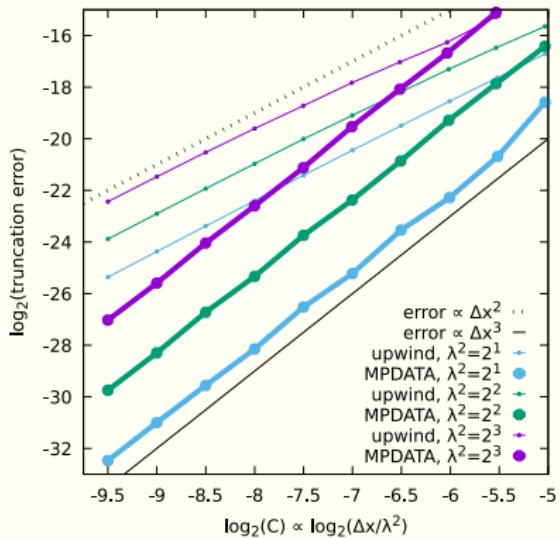
Truncation error as a function of the Courant number  $C = u \frac{\Delta t}{\Delta x}$  which, for fixed  $\lambda^2$ , is proportional to the gridstep.
