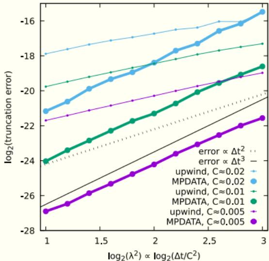
Truncation error as a function of the  $\lambda^2$  parameter which, for fixed  $C$ , is proportional to the timestep.
